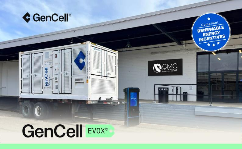
Multipurpose green, grid-independent BRIDGE power - combining hydrogen-fueled generation, software and energy storage for resilient, uninterrupted DC fast charging, backup & 24/7 emergency operations
