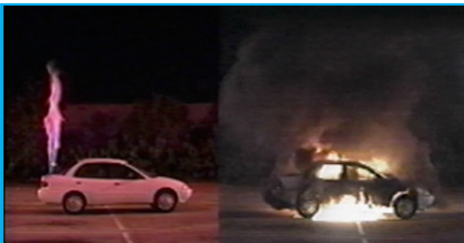
Figure 7: Hydrogen car fire vs. gasoline car fire.
